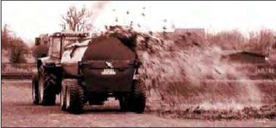
**Figure 2.44: Example of a rotaspreader**
