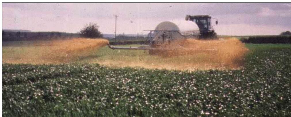
**Figure 2.39: Example of a broadcast technique with low trajectory and low pressure**
