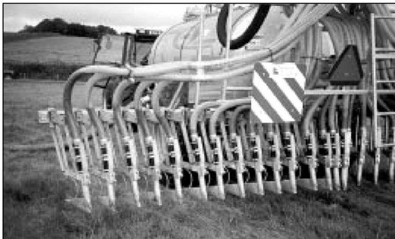
**Figure 2.41: Example of a trailing shoe spreader**
