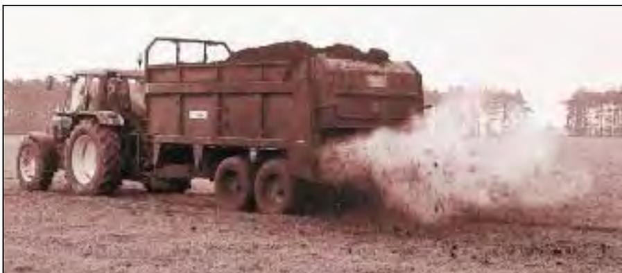
**Figure 2.45: Example of a rear discharge spreader**
