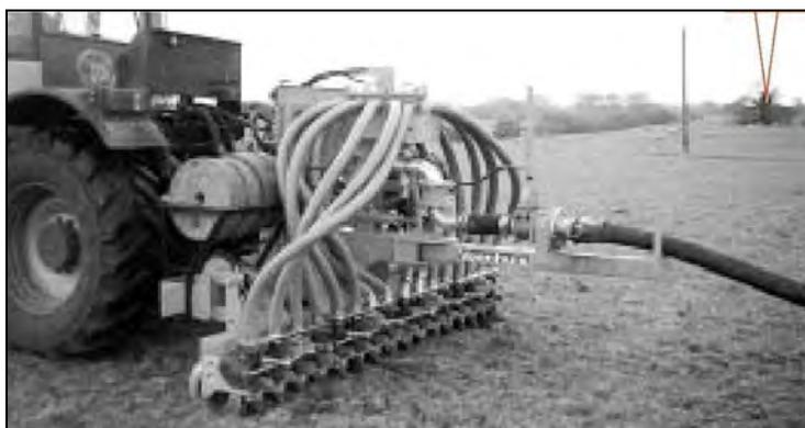
**Figure 2.42: Example of an open-slot shallow injector**
