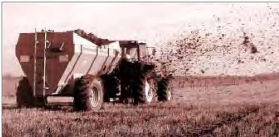
**Figure 2.46: Example of a dual purpose spreader**
