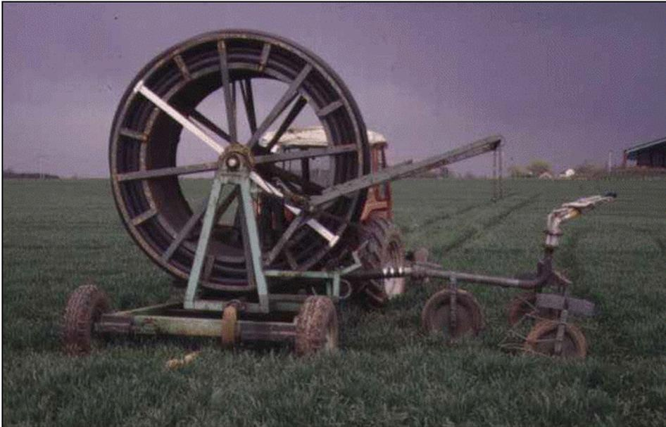
**Figure 2.37: Example of a raingun**
